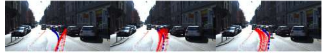
Figure 5. Improved DESIRE-SI prediction samples (red) over iterations. Iterative regression refines the predictions closer to the ground truth future trajectory (blue) matching with scene context.
