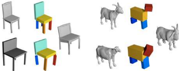
Figure 9: We deform the source mesh (top) to have a shape similar to the target mesh (bottom) by using the inferred primitive representation. Each source mesh point is assigned a local coordinate in the closest primitive’s frame. A deformation of the primitives from the source to target configuration induces a deformed mesh (shown on right).
