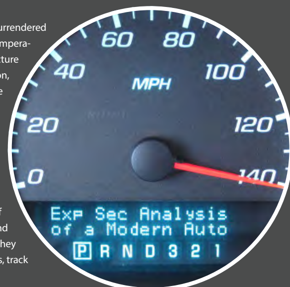
Displaying an arbitrary message and false speedometer reading (note that car is in park)
