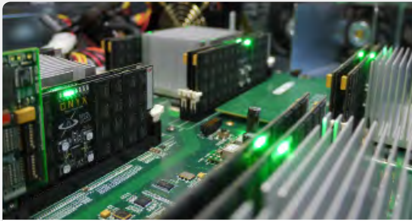
Interior of the Moneta storage array with custom-built Onyx phase change memory modules. It is up to seven times faster than commercial, state-of-the-art solid state drives, and thousands of times faster than conventional hard drives.
